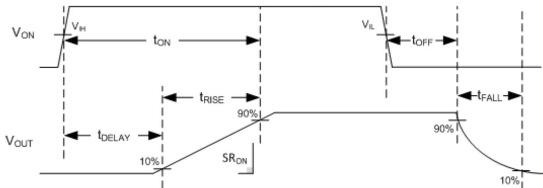
**Figure 32. Timing Waveforms**
