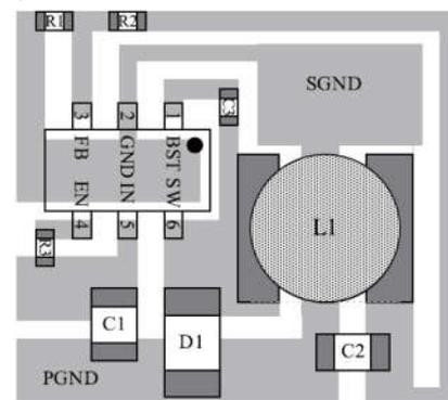
Figure 2: PCB Layout
