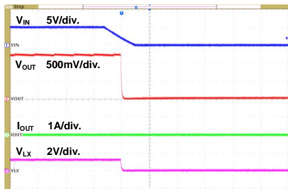
Figure 10. Power Off through VIN Waveform
